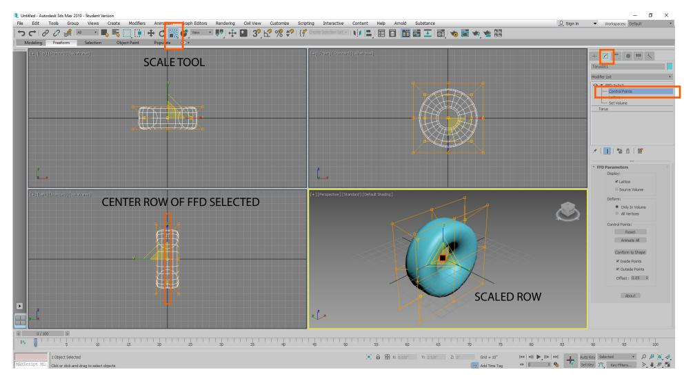
2. Place a FFD 3x3x3 on the torus and select and scale the center row of Control Points and flatten the face of the tire.
