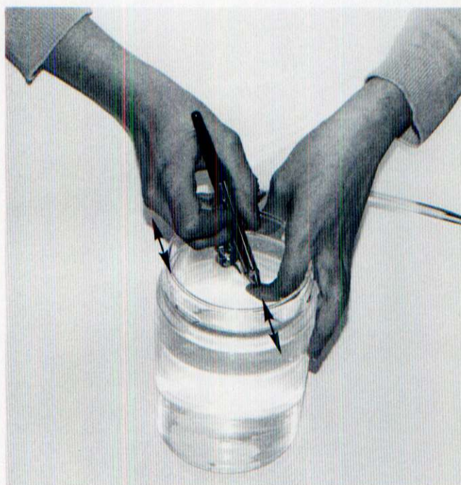
Figure 2-1. To clean the fluid pipe of the airbrush, work the lever with one hand while you alternately block and release the nozzle with the other.
