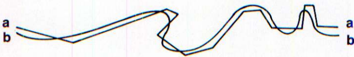
Figure 11-33. Section of the geometrically definable equivalent (a) of a geometrically nondefinable surface (b).
